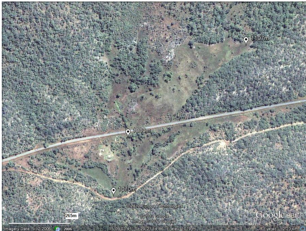
Figure 2 – The Nyabutaye Dambo. The former alignment of the Great East Road crossed the Nyabutaye at its outlet from the dambo (at the 1070m altitude marker). The current alignment cuts the dambo roughly in half. The peat bog occupies most of the open terrain to the north of the road, and is flanked by two semi-permanent streams.
